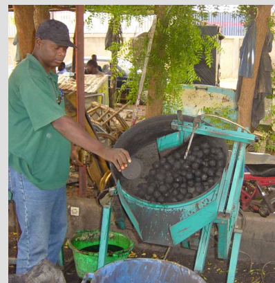
Production of agglomerated briquettes
