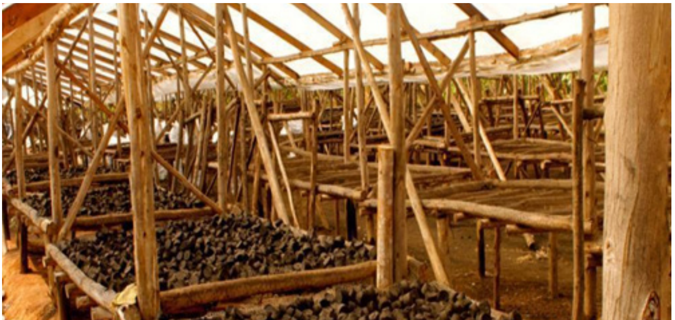
Green Bio Energy briquette sun drying with canopy. Photo: Ziwa Hillington, Green Bio Energy.
