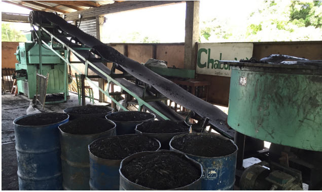
Charcoal briquette production line at Carbon Roots International. Photo: Carbon Roots International
