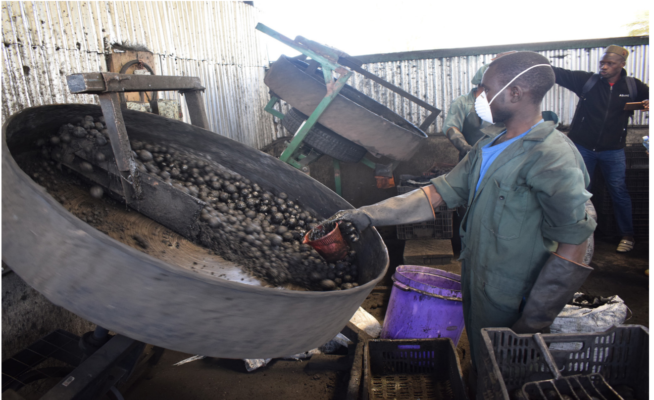
A Sanivation employee operates a briquette agglomerator machine.
